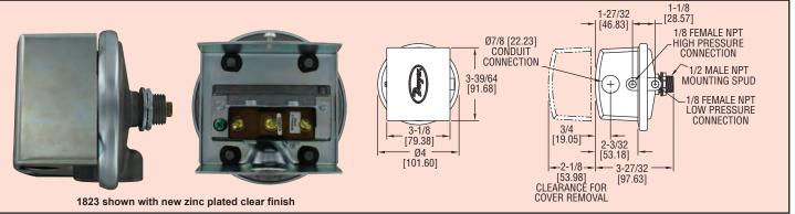
Essential for industrial environments, the Series 1800 combines small size and low price with 2% repeatability for enough accuracy for all but the most demanding applications. Set point adjustment inside the mounting stud permits mounting switch on one side of a wall or panel with adjustment easily accessible on the opposite side. UL and CSA listed, FM approved.
